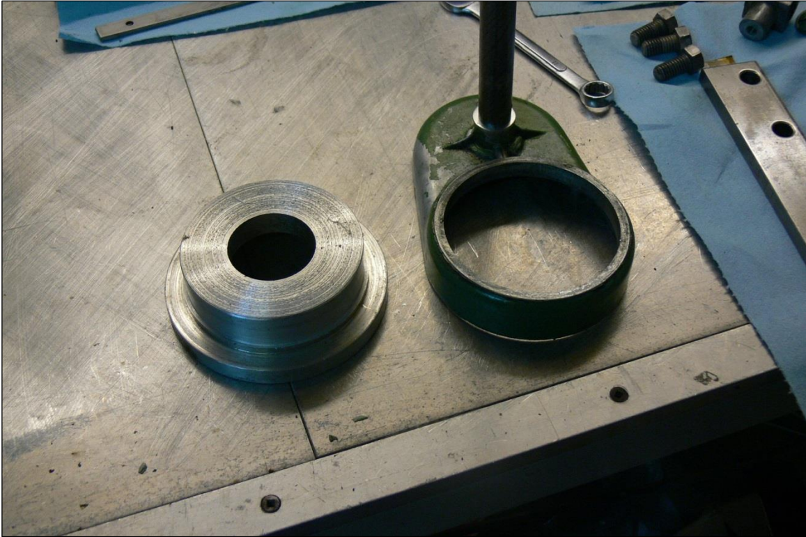
Figure 7 - Aluminum plug to hold casting in the vise
