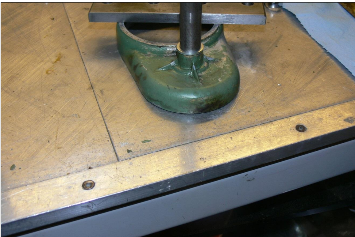
Figure 4 - Casting straight (more-less) after repair
