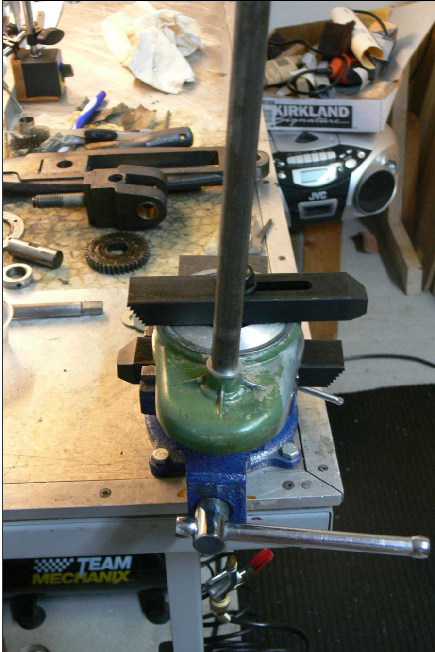
Figure 9 - setup in the vise, ready for heating and straightening
