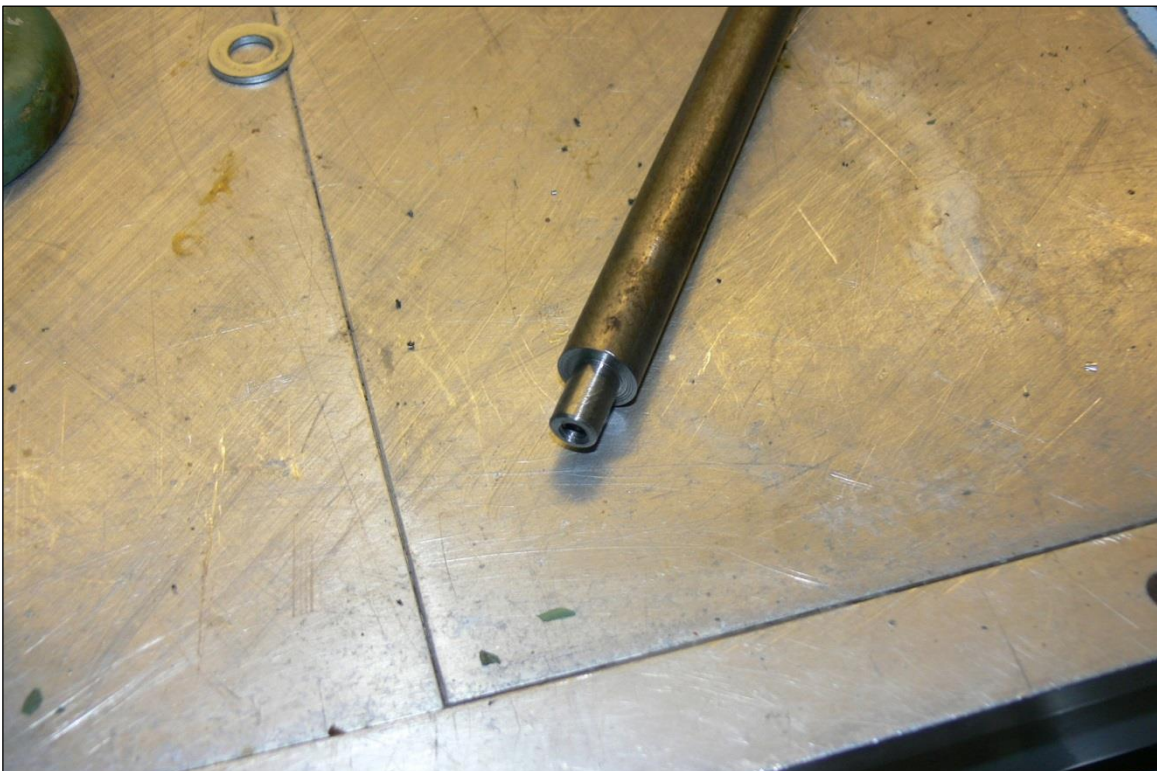
Figure 8 - Steel lever for straightening
