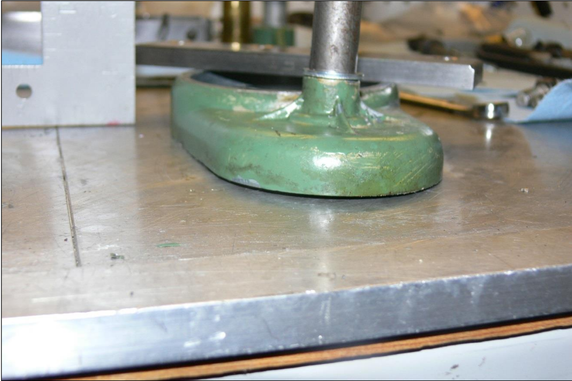
Figure 3 - Casting distorted before repair
